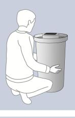
Remove fan housing and thread water pump wire through slit in core pipe. Replace fan housing.
